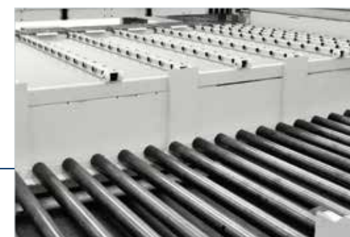
Loading platform High customization and maximum versatility according to the user's requirements, with powered roller conveyor with trilateral loading (opt. on gabbiani gt2).
