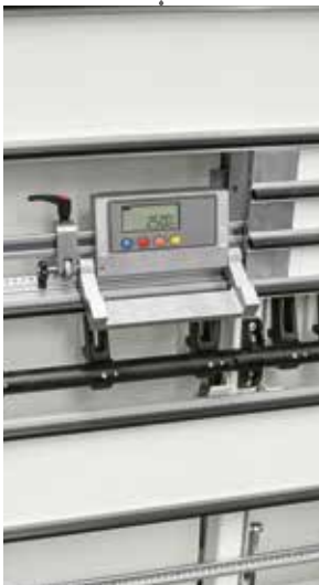
Digital vertical measuring display (opt v, vs, vsi)
