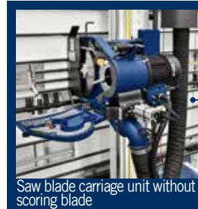
Models with maximum cutting depth from 60 to 80 mm
