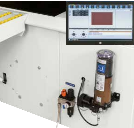
Automatic centralized lubrication managed by the control.
