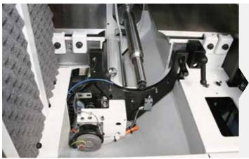
On-board sharpening operations usually take a long time and must be performed by experts. To make these operations simple, fast and precise, on Superset TM the stone automatically moves both axially and radially thanks to an electronic system with speed that can be preset depending on the type of stone/tool and stock removal.
