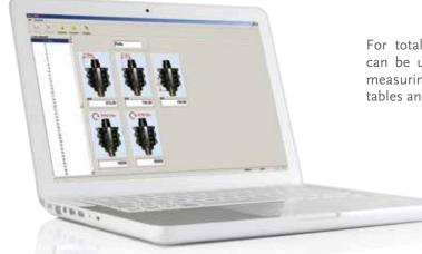
For total process management, the "GT Soft" software can be used to process the data from the projector for measuring tool data, generate new programs, update tool tables and send the information directly to the machine NC.
